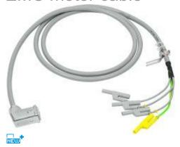
Pre-assembled cable, prepared to connect the asynchronous machine and frequency converter with one another with EMC compliance. The shielded cable has a system plug for connecting to the converter; on the motor side, it is equipped with a shielded terminal and individual 4 mm safety plugs. Set including shield connection adapter for motor. Length 2 m.
